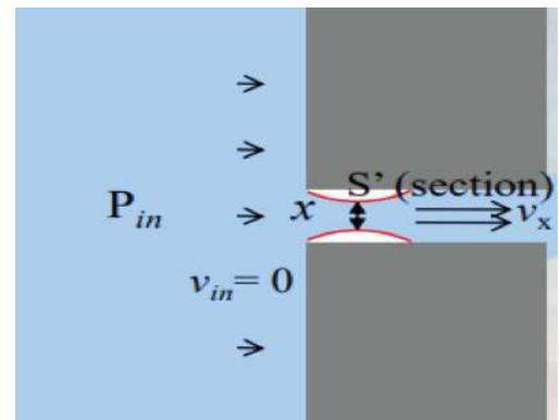
This reduced diameter path is called a “vena contracta” which, on sharp angle cylindrical path, typically reduces the apparent diameter of the hole by 15% to 25%.
