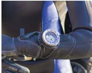
Example: A diving watch will be submitted to a range of pressure from zero differential between inside and outside to the maximum depth specified (ie. 50 m) at temperatures ranging from 60 Celsius to -30 Celsius.
