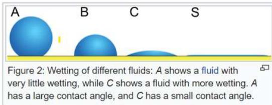
If we take the example of pure water, the contact angle varies a lot depending on materials. Some hydrophobic materials, like Teflon, have a contact angle of more than 90 degrees, some hydrophilic materials, like glass, have a low contact angle.
